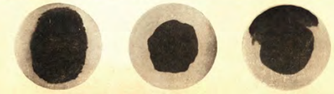
Unretouched X-Ray photographs showing balls with distorted centers
